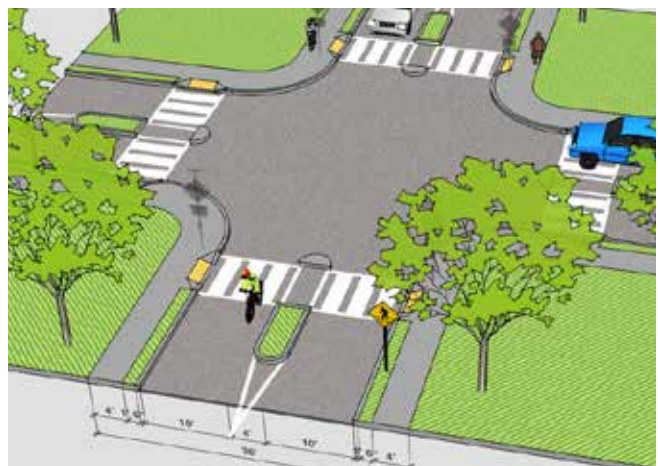
Enhanced crosswalk improvements include standard improvements and can also include medians to make it safer for pedestrians.
