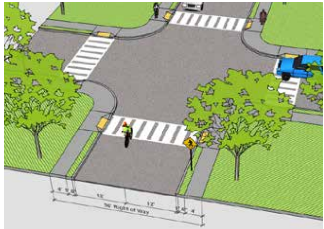
Standard crosswalk improvements include ADA ramps, paint, and signs.
